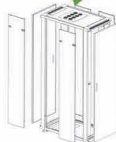
4. Assemble front/rear door and side panel.
