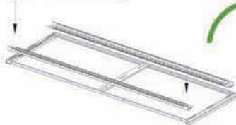
1A. Assemble mounting rail (only width 600mm). (Screw M6x12 & nuts).
