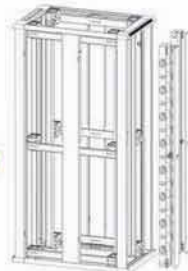
2B. Assemble frame, cable management slot (only width 800mm). (screw M5x10).
